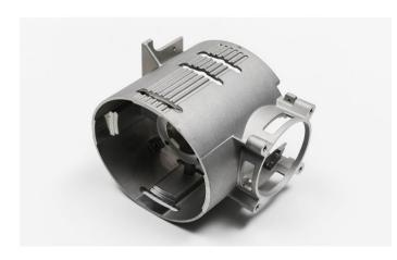
Aluminum 383 (ADC12) is well-suited for casting industrial components due to its unique combination of mechanical properties and casting characteristics. Its high fluidity during the casting process allows for complex industrial components' detailed and intricate molding. It ensures that the final products have precise shapes and dimensions, meeting the stringent requirements often demanded in industrial applications.
